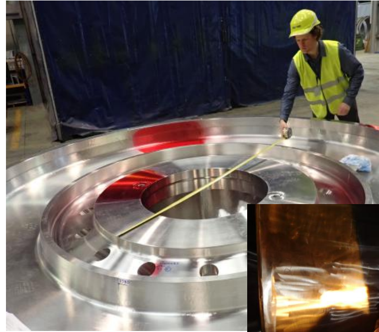
Canyon Ferry Runner Inspection
